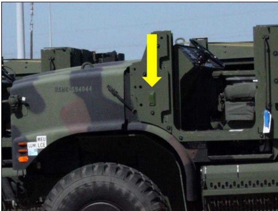
*Omni-ID MaxHD passive RFID tags are being glued to the sides of military vehicles.*
